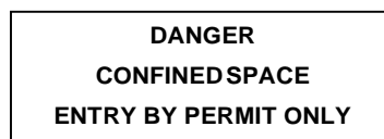
Figure 6: Example of Confined Space Signage Requirements in Canada
